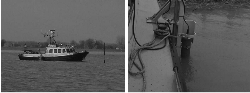
Figure 5.8: The research vessel while measuring flow velocities in the Dutch Upper Rhine in November 1998 (left). The picture on the right shows the ADCP as it is attached to the side of the ship (pictures by Aqua Vision ).
