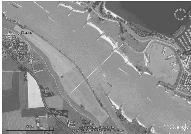
Figure 5.9: An aerial picture of the study area (April 2006, Google Earth). The white line shows the representative transect with a length of approximately 800 m, along which depth and velocity measurements were collected.
